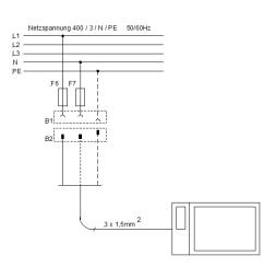
PD 2 G, PD 4 G and PD 2 DG for 230 V Mains connection through CEE plug 7/7 (pre-assembled), all-pole separation from the mains possible.
