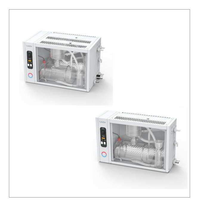
LAUDA Puridest Glass Distillation Apparatus models PD 2 G, PD 4 G, PD 8 G, PD 2 DG and PD 4 DG produce ultrapure, bacteria and pyrogen-free distillate with a very low conductivity (approx 2.2  $\mu$ S/cm at 25 °C for mono distillate and 1.6  $\mu$ S/cm at 25 °C for bi distillate). The distillate is in conformity with DAB regulations and the regulations of international pharmacopoeia.
