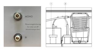
① Float switch mono stage② Float switch bi stage
