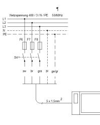
PD 8 G and PD 4 DG Permanent mains connection through on-site switch S4, all-pole separation from the mains possible.
