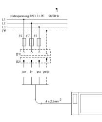
PD 8 G and PD 4 DG Permanent mains connection through CEE plug according to IEC standard 60309-2, all-pole separation from the mains possible.
