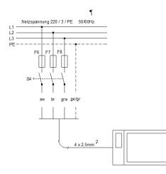
PD 8 G and PD 4 DG Permanent mains connection through on-site switch S4, all-pole separation from the mains possible.
